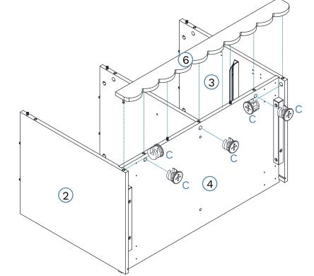
Attach panel [6] to step 8 assemble the piece and secure with 5 x cams (C).
