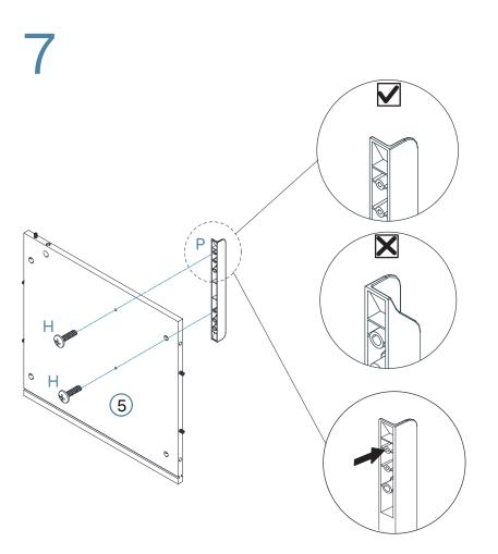
Attach 1 x rail track (P) to panel [5] and secure with 2 x screws (H).
