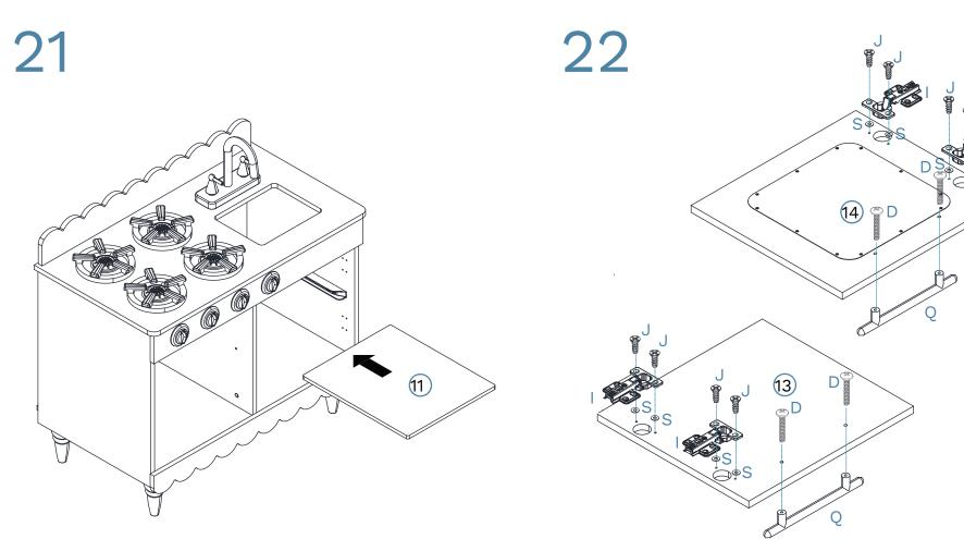
Insert panel [11] to step 20 assemble the piece as shown.
