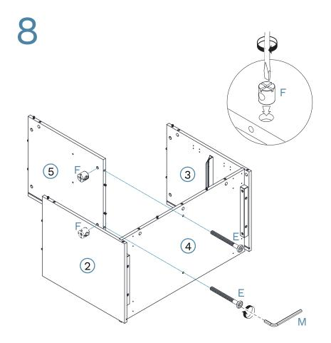
Insert 2 x nuts (F) to panel [5] as shown.Attach panel [5] to panel [4] and secure with 2 x screws (E) and allen key (M).
