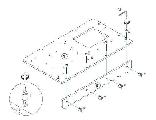
Insert 4 x nuts (F) to panel [10] as shown. Attach panel [10] to panel [1] and secure with 4 x screws (E) and allen key (M).
