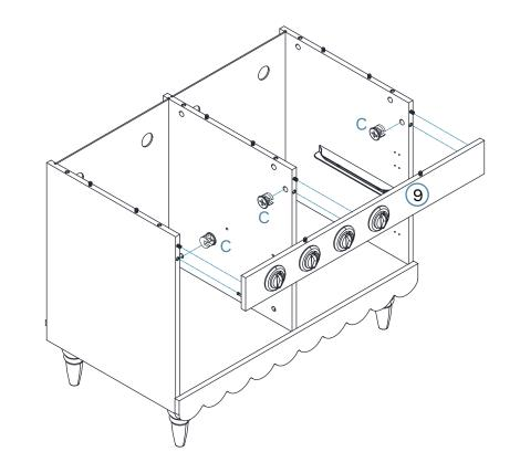
Attach panel [9] to step 13 assemble the piece and secure with 3 x cams (C).
