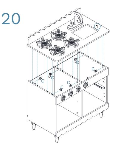
Attach 1 x tap (T) to panel [1] and secure with 2 x screws (N) and 2 x washer (K). Tighten with an Allen Key (M). Assemble 4 x burners (R) as shown. Attach 4 x burners (R) to panel [1] and secure with 12 x screws (L). Tighten with a screwdriver.
