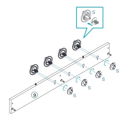
Attach 4 x switches (S) into panel [9], in order to guarantee the switches move smoothly, do not lock the rotary knob tightly.
